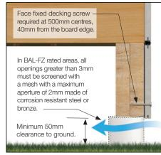
FIGURE 4 BOTTOM FINISH AND CLEARANCE
