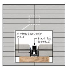
FIGURE 6 OPTION 2: SQUARE PANELLED JOINTS
