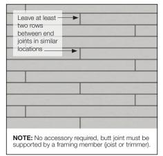
FIGURE 5 OPTION 1: CONTINUOUS (STAGGERED) JOINTS
