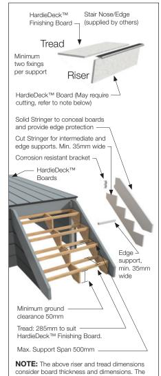
resulting riser and going must be within 115-190mm and 240-355 mm, respectively.
