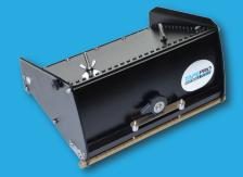
The Tapepro T2 Flat Boxes are designed to apply joint compound to all flat recess and butt joints, automatically crowning the joint and feathering the edges. The coat thinkness is controlled by a cam adjuster on the front of the box; more spring pressure results in a lighter coat.
